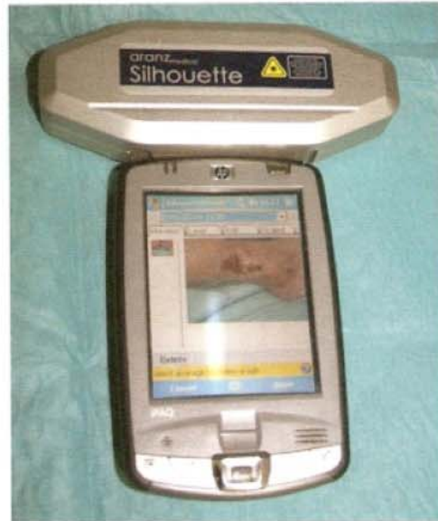
Fig. 11.1 Portable laser scanner for digital wound image analysis
