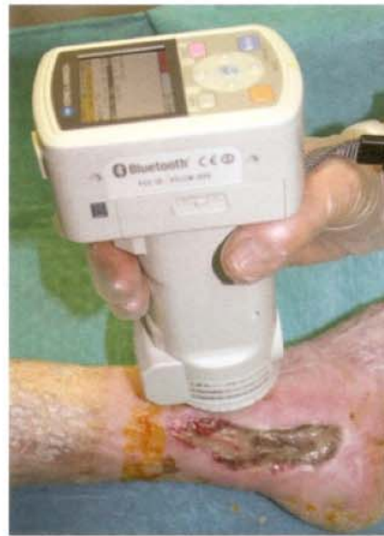
Fig. 11.2 Non invasive tristimulus colorimeter for wound bed color assessment
