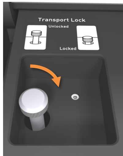
Figure 9: Locking the Plate Carrier
