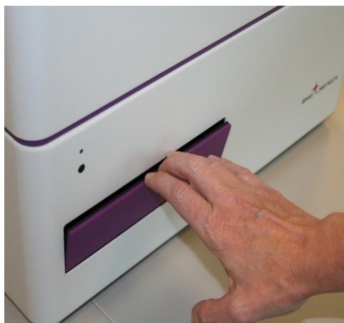
Figure 24 : With a fingernail, open the plate carrier door and see if the plate carrier is locked by gently trying to move it
